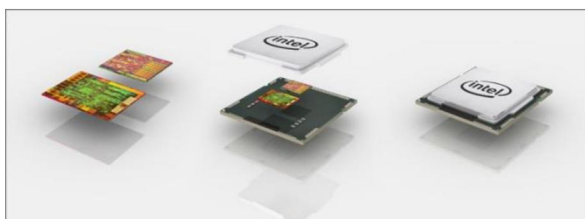
Figure 4. Processor housing assembly
