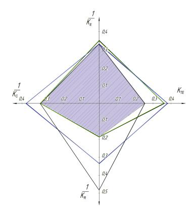
$K_R$  – coefficient of resistance to tripping;  $K_E$  – endurance coefficient;  $K_C$  – coupling coefficient;  $K_{TE}$  – technical and economic coefficient
