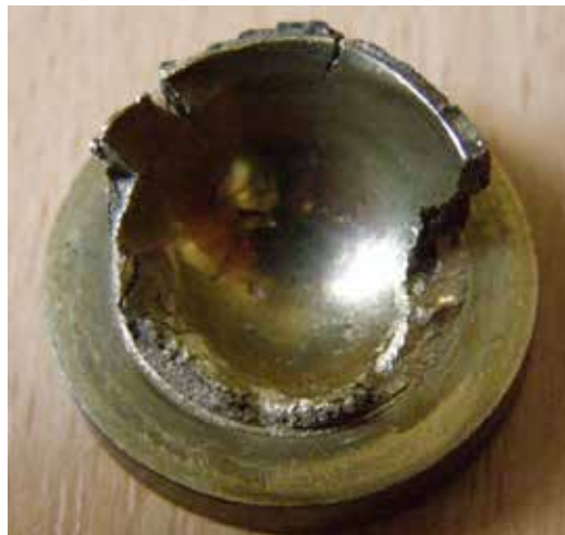
Fig. 5. Heel separation from the plunger bore
