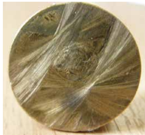
Fig. 4. Complete wear of the heel ring support with rolling of the hydrostatic bearing hole
