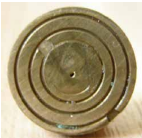
Fig. 3. Common type of plunger heel wear
